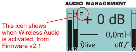
This icon shows when Wireless Audio is activated, from Firmware v2.1
